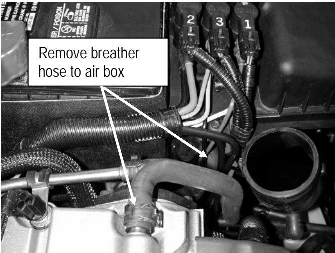
e) Remove the breather hose going to the air box. Check for oil. If present, clean as necessary.
